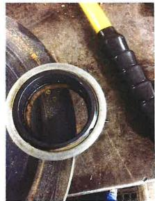
Rotating element for the mechanical seal is bad,
