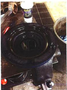
Oil in poor condition, metal particles in the oil.
