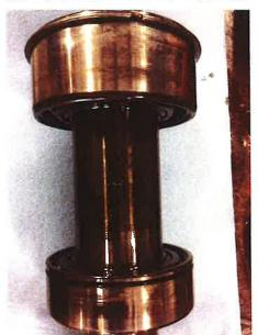
Bearings show damage from spinning inside the housing from lack of proper Lubrication and excessive heat build up.
