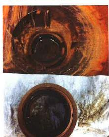
Mechanical seal plate is ok, the mechanical seal is bad.
