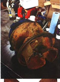
Rotating assembly pulled from pump #2 station #5. The impeller is in very bad worn condition. The bearing cavity oil was in very poor condition. The mechanical seals are leaking, water in the seal cavity oil.
