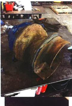
Rotating assembly pulled from Pump #1 station #5. The impeller is very bad worn condition. The bearing cavity oil was in extremely poor condition. The mechanical seal cavity oil had a large amount of water mixed in with the oil.
