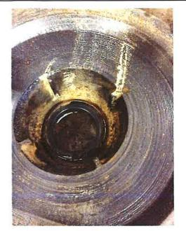
Seal plate is ok. The mechanical seal is bad.
