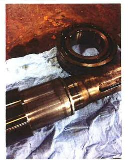
Outboard bearing shaft fit is ok.
