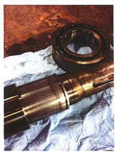
Shaft is ok at the bearing fit for theminvoard bearing
