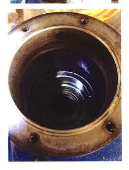
Inboard bearing had spun in the bearing housing.
